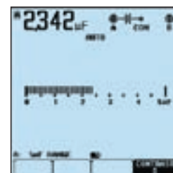
Check the starting capacitor of a motor with the ScopeMeter 124
