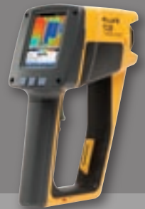
Fluke Ti20 Thermal Imager
