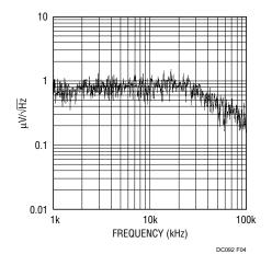
Figure 4. Output Spot Noise 1kHz to 100kHz
