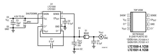
Figure 1.DC092 Schematic (-4.1V Generator)
