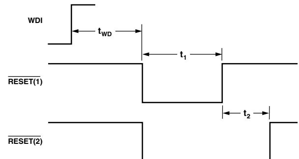
Figure 8. Watchdog  $\overline{RESET}$  Timing
