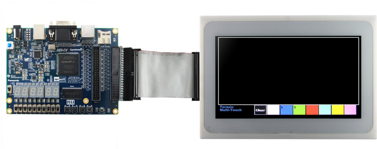
Figure 5-7 Hardware Setup with DE0-CV
