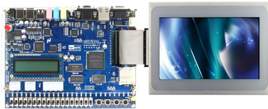
Figure 5-8 Hardware Setup with DE2-115
