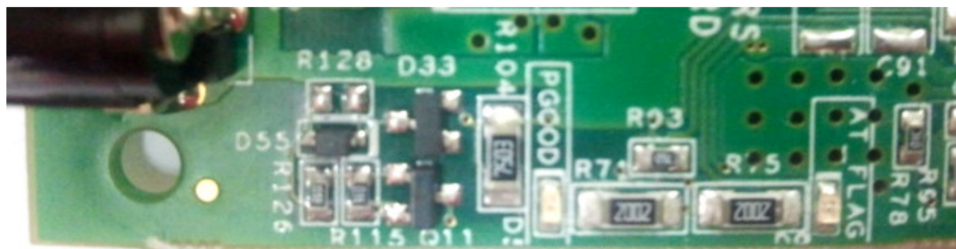
Figure 5: Power_Good LED Indication D5
