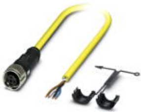
Sensor/Actuator cable, 4-position, PVC, yellow RAL 1021, free cable end, on Socket straight M12 SPEEDCON, A-coded, Cable length: 0.5 m
