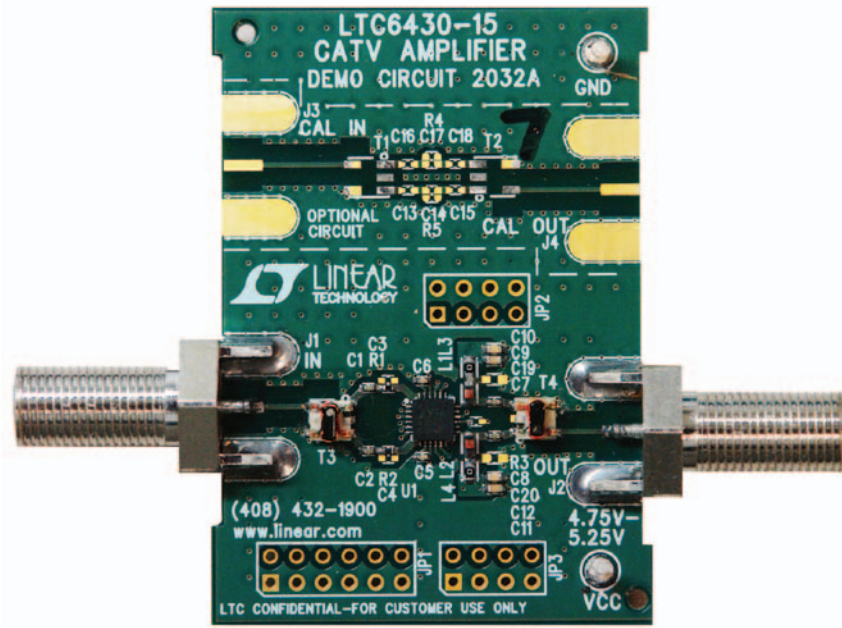
Figure 17. LTC6430-15 CATV Evaluation Board
