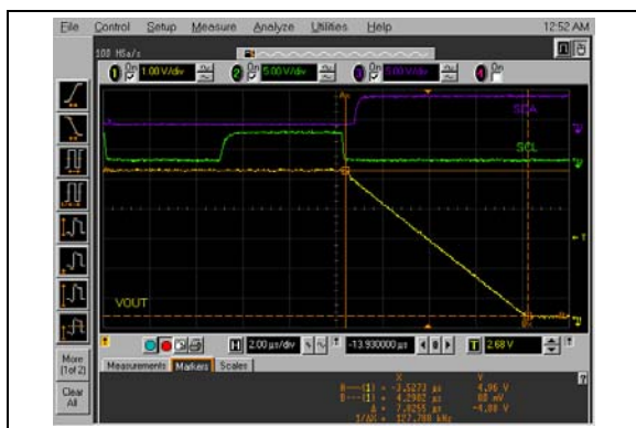
FIGURE 2-97: Full-Scale Settling Time (FFFh to 000h) (MCP4726).
