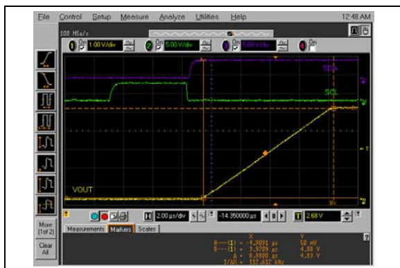
FIGURE 2-96: Full-Scale Settling Time (000h to FFFh) (MCP4726).
