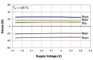
Switch Points vs Supply Voltage
