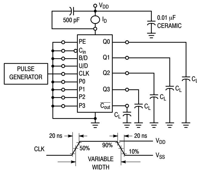
Figure 1. Power Dissipation Test Circuit and Waveform
