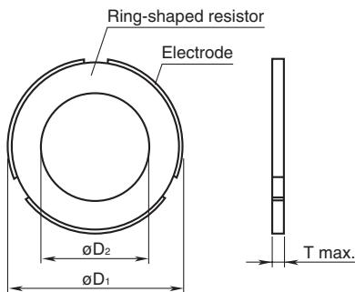
**SIDE SURFACE ELECTRODE TYPE(6-ELECTRODE)**
