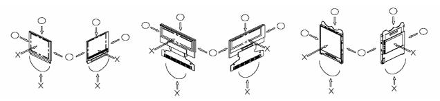
(7) Do not apply stress to the LSI chips and the surrounding molded sections.
