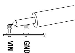
Figure 2. Measuring Input or Output Ripple
