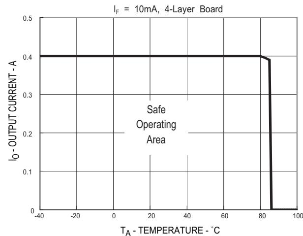
Figure 3. Maximum Output Current Rating vs Ambient Temperature
