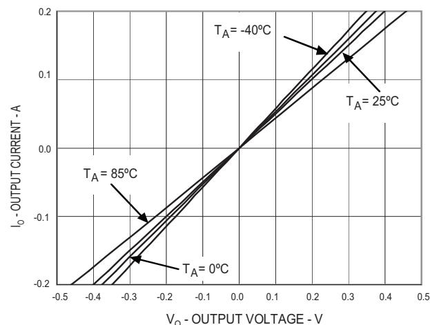
**Figure 9. Typical Output Current vs Output Voltage**
