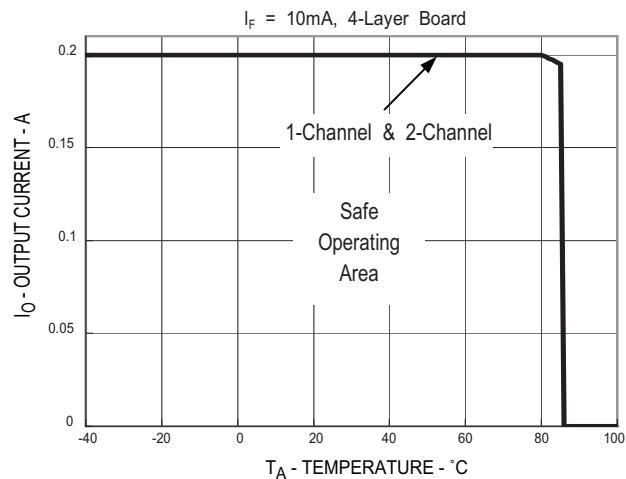
Figure 4. Maximum Output Current Rating vs Ambient Temperature
