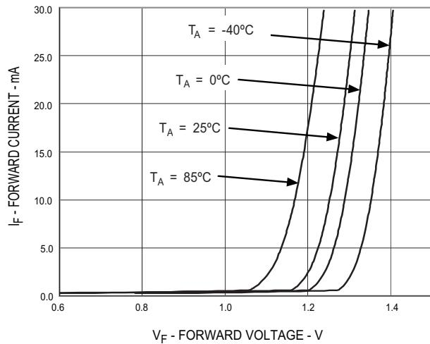
**Figure 7. Typical Forward Current vs Forward Voltage**
