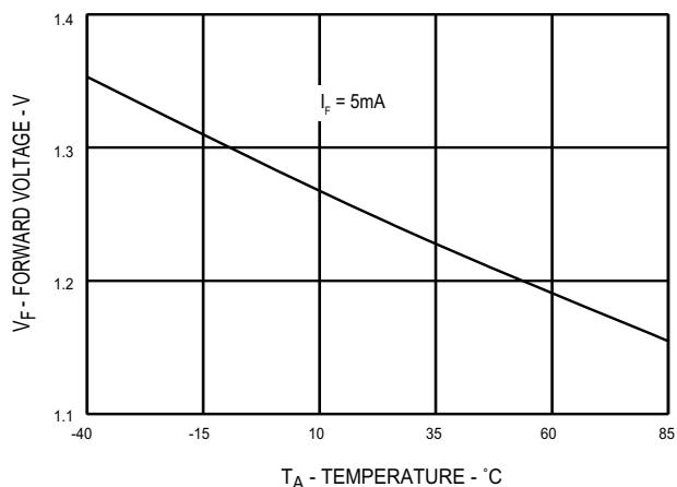
**Figure 6. Typical Forward Voltage vs Temperature**
