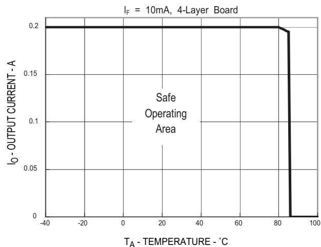
Figure 2. Maximum Output Current Rating vs Ambient Temperature
