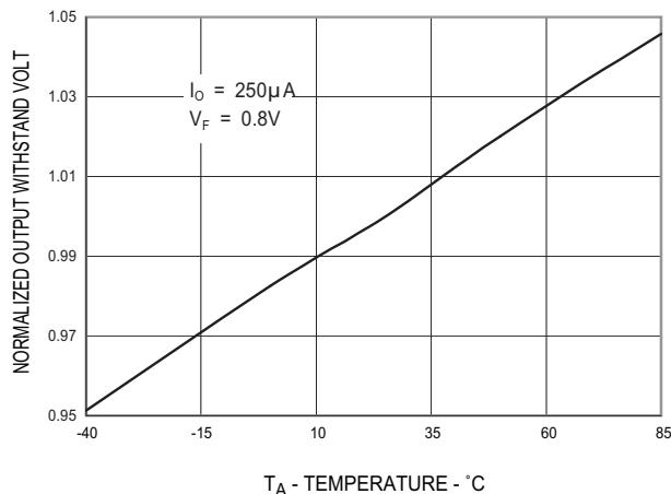
**Figure 5. Normalized Output Withstand Voltage vs Temperature**
