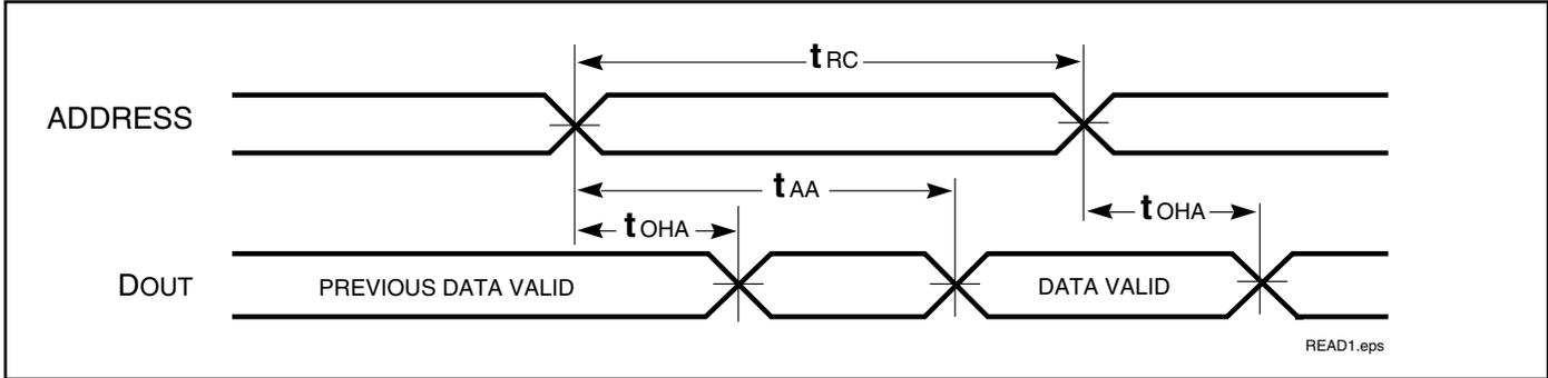
**READ CYCLE NO. 2<sup>(1,3)</sup>** ( $\overline{CE}$  and  $\overline{OE}$  Controlled)
