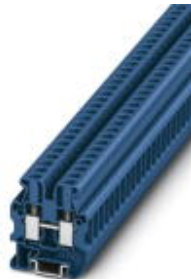
Mini feed-through terminal block, Connection method: Screw connection, Cross section: 0.2 mm 2 - 4 mm 2 , AWG: 24 - 12, Width: 5.2 mm, Color: blue, Mounting type: NS 15
