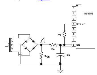
FIGURE 9. ADDING SLOPE COMPENSATION
