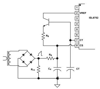
FIGURE 10. ADDING SLOPE COMPENSATION USING CT
