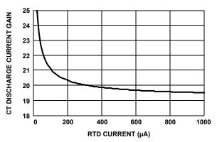
FIGURE 5. CT DISCHARGE CURRENT GAIN vs RTD CURRENT
