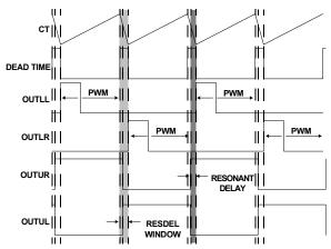
FIGURE 11. BRIDGE DRIVE SIGNAL TIMING
