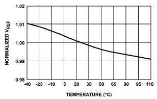
FIGURE 4. REFERENCE VOLTAGE vs TEMPERATURE
