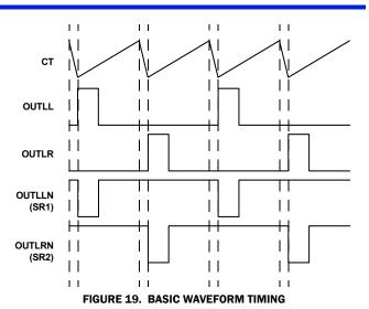
Referring to Figure 19, the SRs alternate between being both on during the free-wheeling portion of the cycle (OUTLL/LR off) and one or the other being off when OUTLL or OUTLR is on. If OUTLL is on, its corresponding SR must also be on, indicating that OUTLRN is the correct SR control signal. Likewise, if OUTLR is on, its corresponding SR must also be on, indicating that OUTLLN is the
