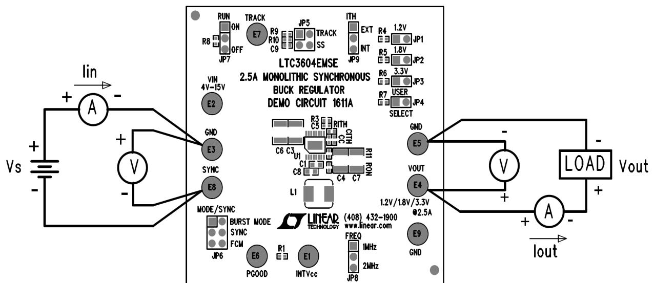
Figure 1. Proper Equipment Measurement Set-Up
