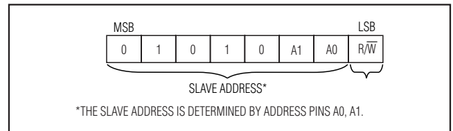
Figure 2. DS3501 Slave Address Byte
