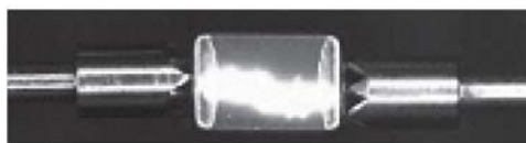
Standard Capacitor with Surface Arc-over
