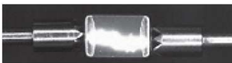
Standard Capacitor with Surface Arc-over
