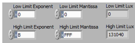
Figure 15. Registers x02 and x03 Lux Limit Controls
