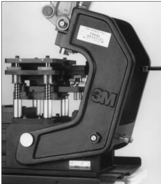
Figure 3. Press leaned back
