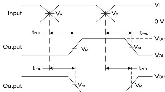
**Voltage Waveform Propagation Delay Times
