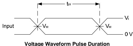
**Voltage Waveform Pulse Duration**
