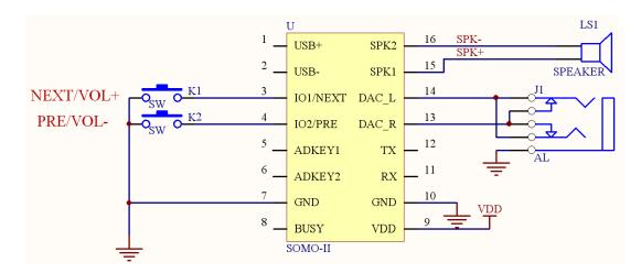
This is an example schematic showing the simplest connections to the SOMO-II for KEY MODE. Only 2 buttons are required. NEXT/VOL+ will start playing a track if currently stopped, and will raise the volume if the button is held down for > 1.2 seconds. PRE/VOL- will start playing a track if currently stopped also, and will lower the volume if the button is held down for > 1.2 seconds. See the table in Section 5.3 for more information.
