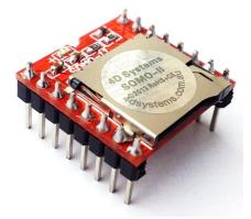
The SOMO-II features an on board 16bit MCU, specifically designed for hardware audio decoding.
