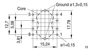
Hole arrangement View in mounting direction
