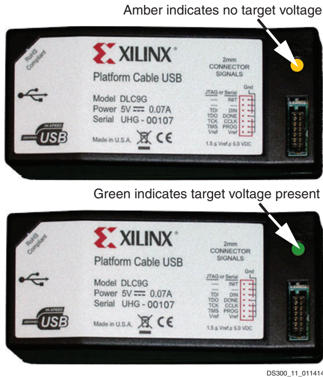
Figure 11: Status LEDs Indicating Target Voltage
