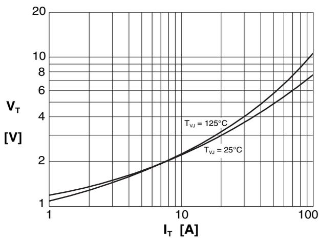
Fig. 3 On-state voltage
