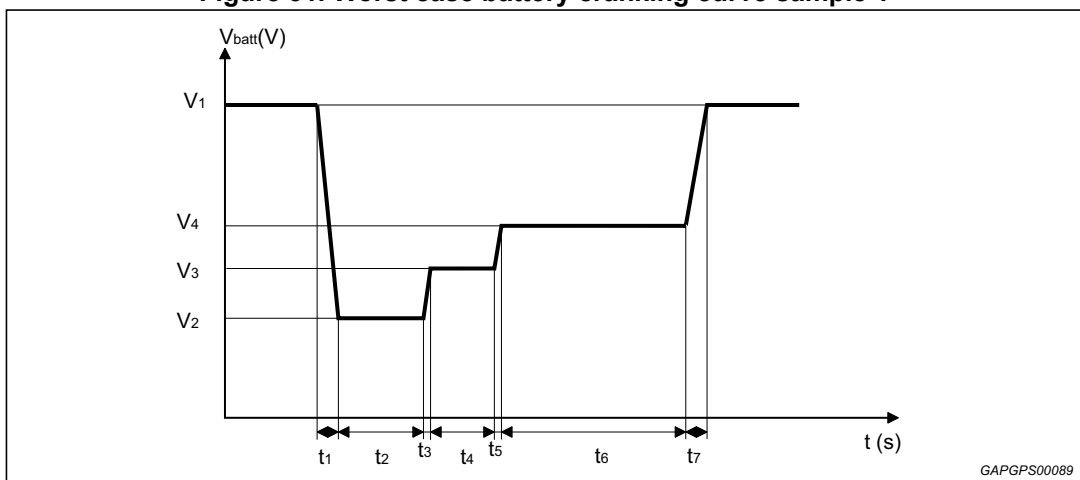
Figure 31. Worst case battery cranking curve sample 1
