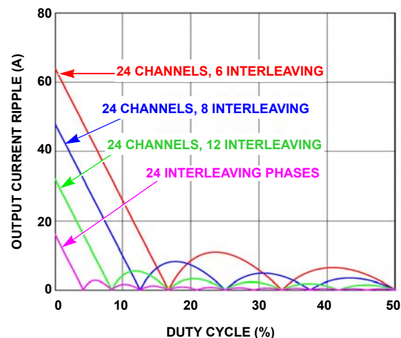
FIGURE 17. OUTPUT CURRENT RIPPLE vs DUTY CYCLE, PHASE COUNT
