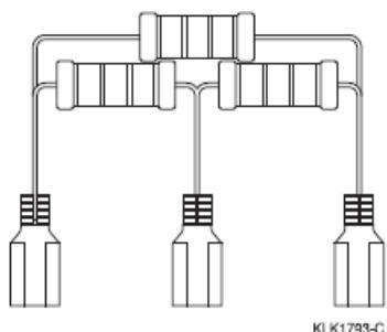
**Three-phase capacitors –  $V_R = 220$  V AC, 50/60 Hz, delta connection**
