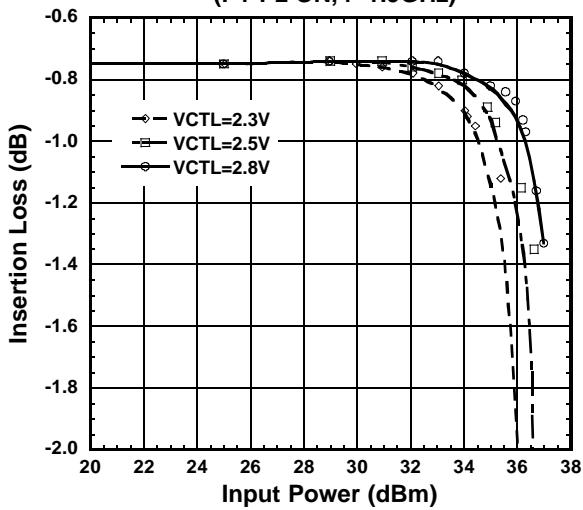
**Insertion Loss vs. Input Power**
