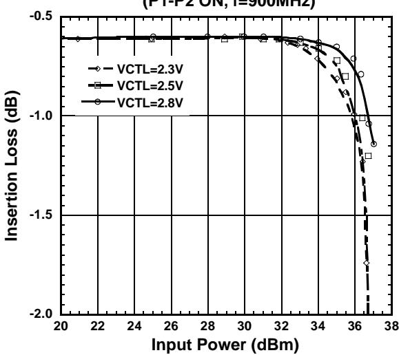
**Insertion Loss vs. Input Power
