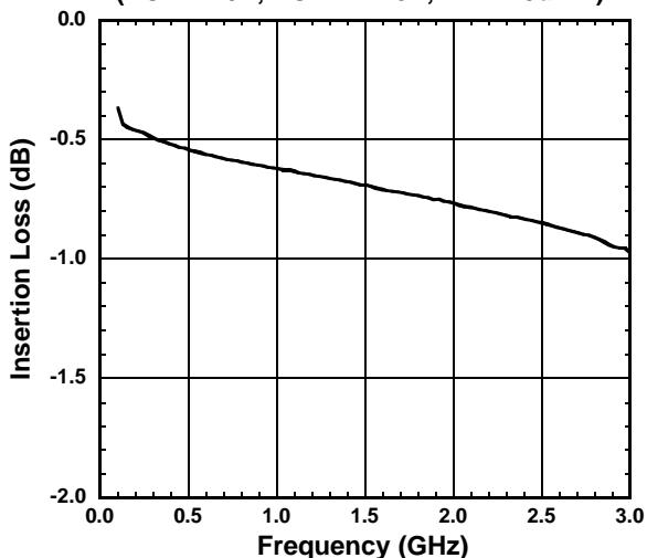
**P3-P4 Insertion Loss vs.Frequency**
