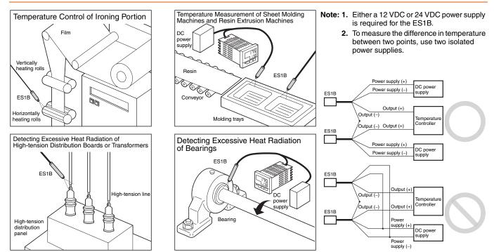
Do not use the Infrared Thermosensor in locations where the ambient temperature changes rapidly. To use the Infrared Thermosensor in locations subject to rapid changes in temperature due to radiant heat or movement of hot air, use a heat shield or other method to reduce rapid changes in temperature as much as possible.
