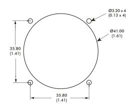
The joystick is dropped into the panel cut-out. The joystick and boot must be kept in place by bezel (option 6 & 7). For panel thickness of <3mm, M3 x 16 countersunk machine screws are recommended. To ensure a good panel seal, gaskets are available as an optional extra.
