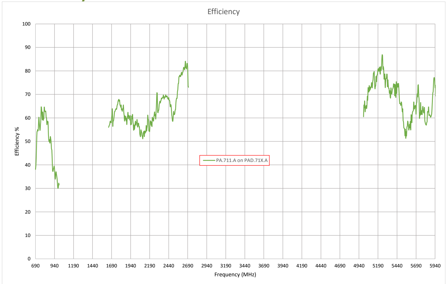
Figure 8. Efficiency of the PA.711.A LTE Antenna on MIMO PAD.71X.A
