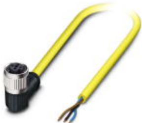
Sensor/Actuator cable, 3-position, PVC, Yellow RAL 1021, Free cable end, on Socket angled M12-SPEEDCON, A-coded, Cable length: 10 m
