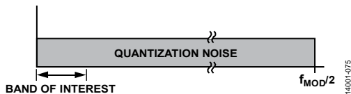
Figure 69. \Sigma - \Delta ADC Quantization Noise (Linear Scale X-Axis)
