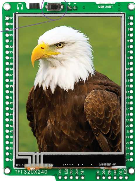
Figure 4-2: Frontal reset button
