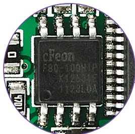
Figure 11-1: Flash memory module
