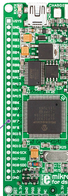
Most microcontroller pins are available for further connectivity via two 1x26 rows of connection pads on both sides of the mikromedia board. They are designed to match additional shields, such as Battery Boost shield, Gaming, PROTO shield and others.
