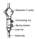
Note: 1. The spring washer comes with the lock nut.
