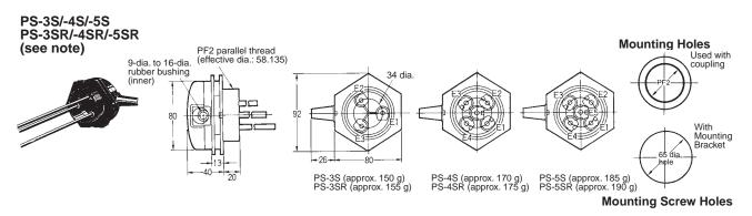
Note: The PS-3SR, PS-4SR, and PS-5SR have built-in resistor of 6.8 k $\Omega$  and used for the two-wire 61F models.
