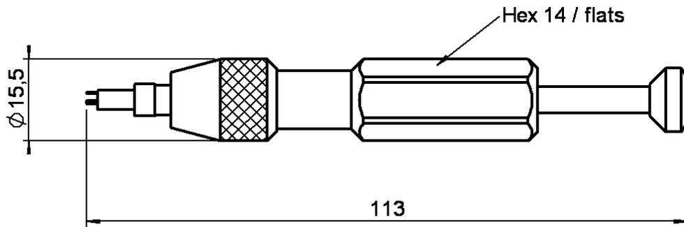
Unscrew the 2 half bodies to remove the front part R282.920.110 .
