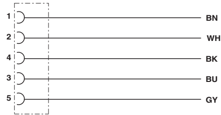
Contact assignment of the M12 socket
