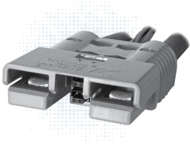
SBX® and SBE® connectors can integrate up to 8 auxiliary power / signal contacts along with the two primary power circuits. SBE® connectors feature an IEC 60950 touch safe housing molded from a chemical resistant PBT/PC blend resin. SBX® are molded from a rugged PC resin and are rated IP20 per IEC 60529.
