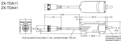
Vinyl-insulated round cable 5.2 dia. 10 conductors, (conductor crosssection: 0.09 mm², insulator diameter: 0.7-mm dia.), standard length: 2 m
