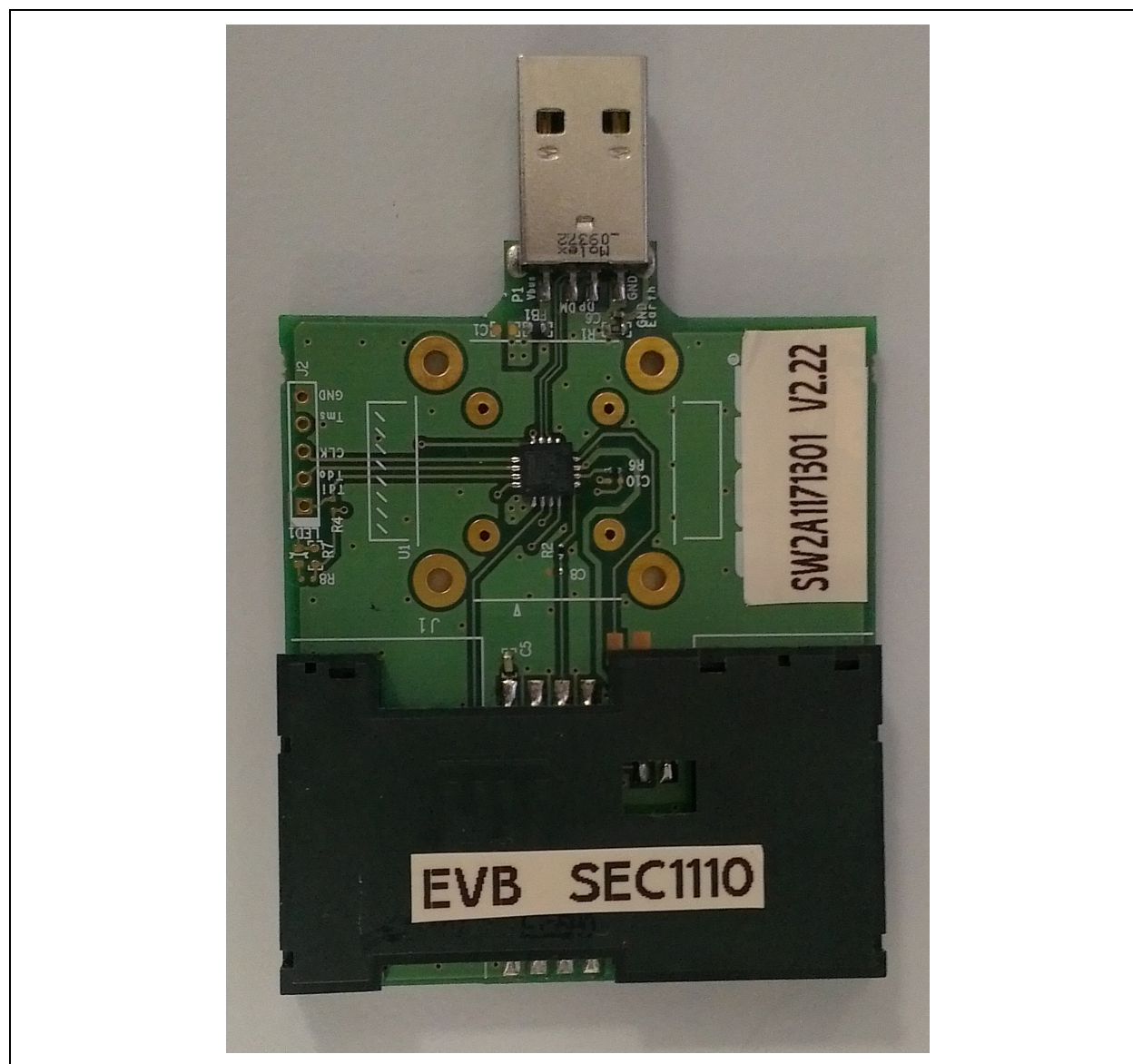
FIGURE 2-6: EVB-SEC1110 COMPONENT SIDE TOP LAYER
