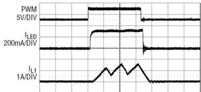
Figure 2. DC1279A 30V LED string PWM Dim, PVIN=12V
