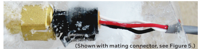
Figure 2. PX3 Series External Freeze/Thaw Resistance
