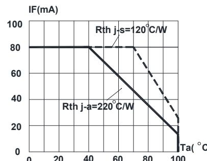
FIG.5 MAXIMUM FORWARD DC CURRENT VS AMBIENT
