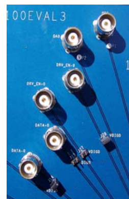
FIGURE 5. HIGH SPEED, TESTER SIDE, DRIVER CONNECTIONS
